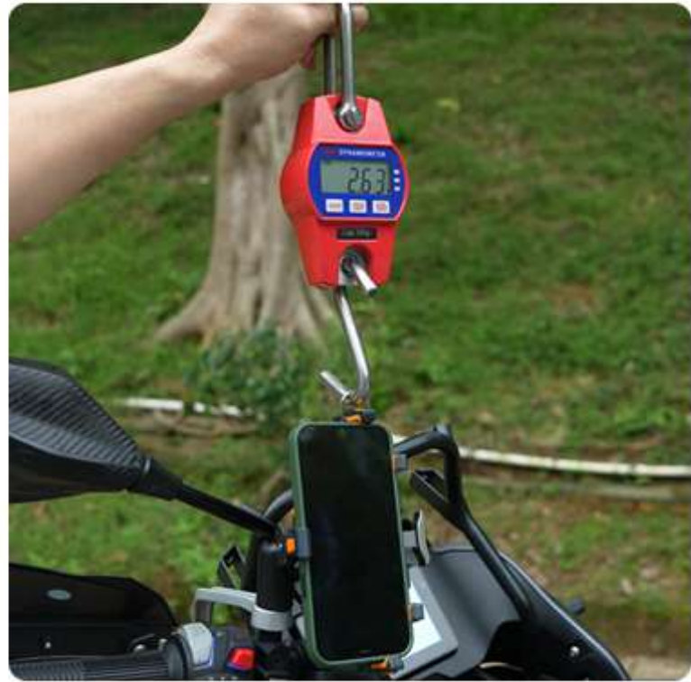
Mechanical Traction Structures Pull Testing
